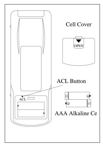
Remote controller battery requirements: Two AAA alkaline cells.
